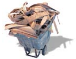
Typical broadloom installation waste: 8-12%
